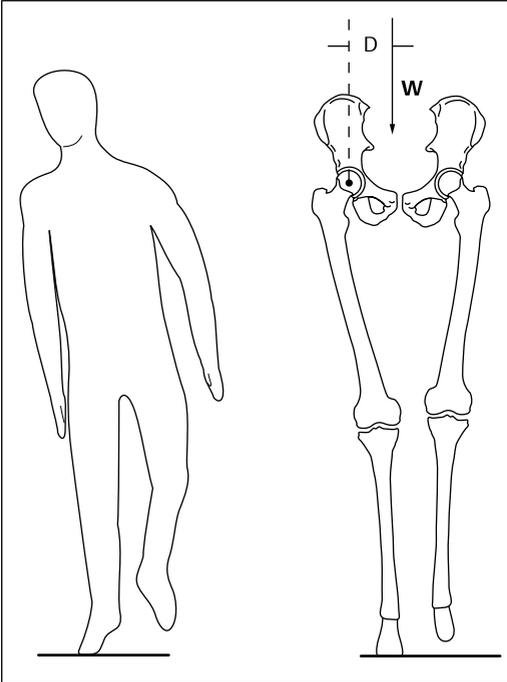
Fig. 9.4 Effect of the Duchenne limp on the loading of the hip joint. Shifting the body mass to the side of the standing leg decreases the moment arm of the gravitational force  $W$ . Consequently the muscle force required for equilibrium decreases as well. Due to the decrease in muscle force, the load on the hip joint decreases.
