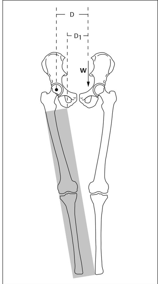
Fig. 9.5 Influence of an orthosis on the load on the hip joint. The orthosis shifts the center of rotation from the center of the femoral head to the point of support at the tuber ischiadicum. This shift decreases the moment arm of the gravitational force  $W$  from  $D$  to  $D_1$ . Due to the changed moment arm, the muscle force, and hence the joint load, decrease as well.
